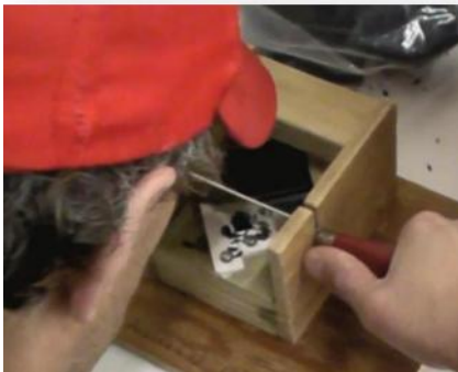
Shaving corners off commercially produced square plastic caps
