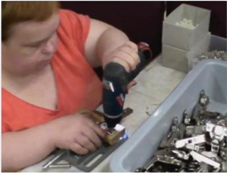
Shaped wooden block and vise to connect plastic dowels to cabinet hinges
